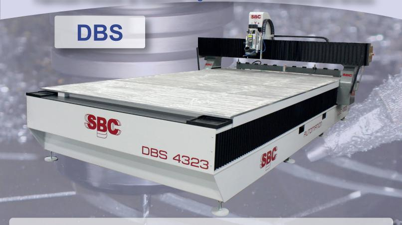
The DBS milling center is a fully bellow-protected DBE version, designed for machining extremely dusty technical parts such as composites, but also works with with plastics, wood, aluminium, brass ....
